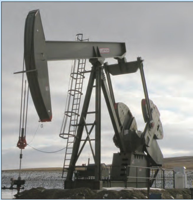
A Lufkin conventional crank balanced pumping unit, a "work horse" of the oil patch, extracting Bakken crude oil in McKenzie County, N.D.
