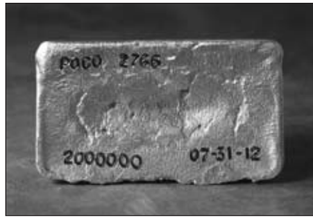
This 744-troy-ounce bar contains the 2,000,000th ounce of gold poured at Pogo and is roughly 93.6 percent gold.
