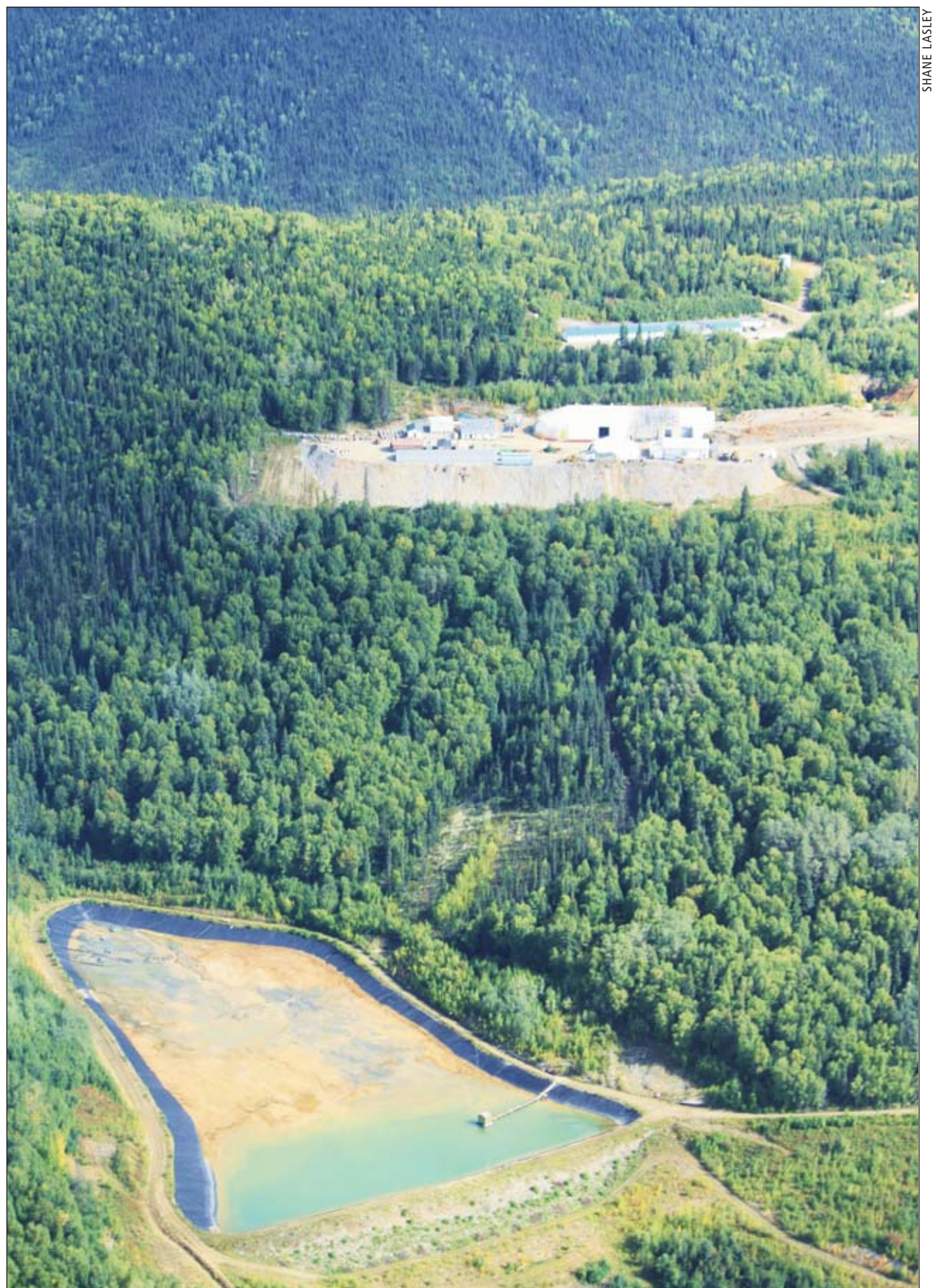
Fire River Gold plans to reprocess 100 metric tons per day of tailings from historic mining at Nixon Fork. It is estimated that the 140,000 metric tons of tailings average more than 7.5 g/t.
