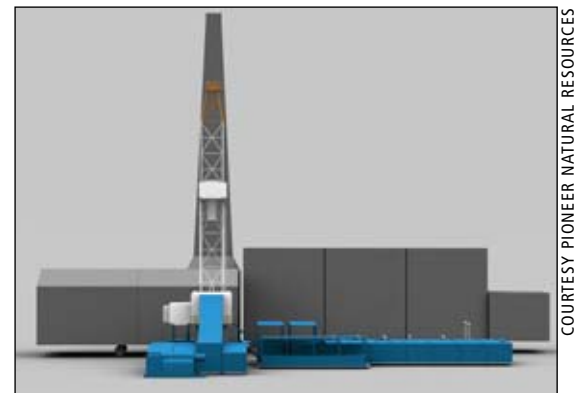
The Arctic Fox No. 1 drilling rig being built for use by Pioneer Natural Resources will have an in-line layout that breaks down into 35 truckable loads.
