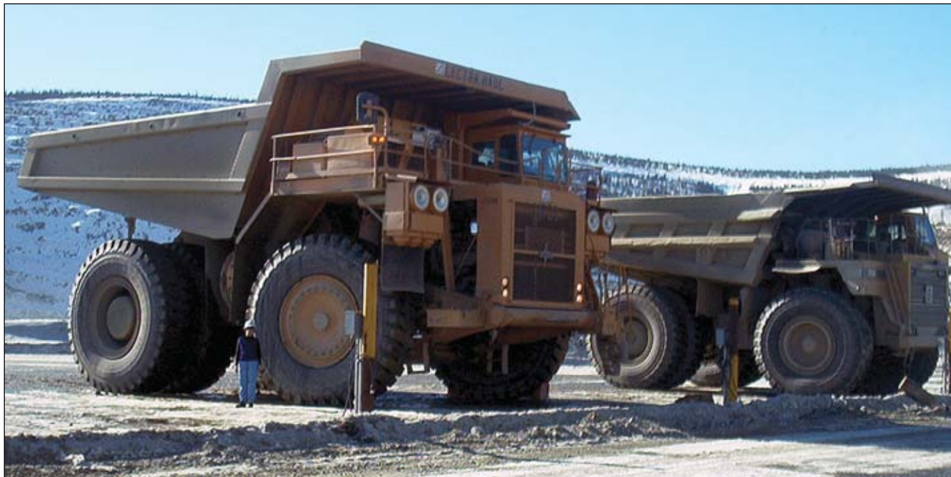
Six new haul trucks, similar to the truck pictured at left, are due to be delivered to Fort Knox in late July or early August. The six Caterpillar 789 haul trucks each provide a 190-ton capacity. The new trucks dwarf the mine's 150-ton trucks, pictured at right.
