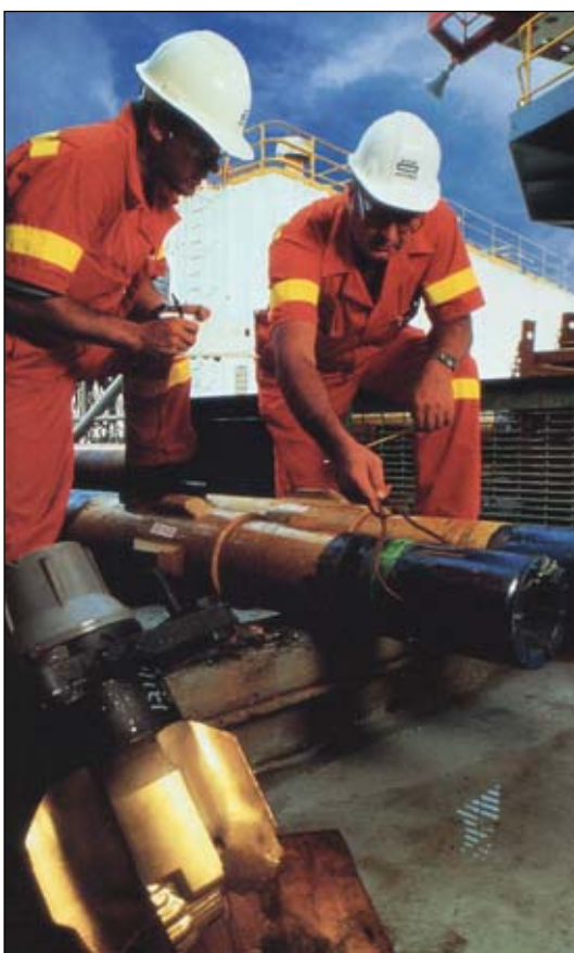
Baker Hughes workers measure the outer diameter of a mud motor. Baker Hughes supports projects of all sizes, with people experienced in every phase of well construction and maintenance, industry-leading technology and a world-wide service network. Baker Hughes INTEQ serves as the focal point for integrated solutions involving more than one Baker Hughes company.
