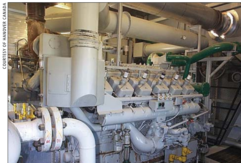
A typical lease package from Hanover Canada. This particular three-stage package includes a Waukehsa 5790GL driver (1215 HP) with Ariel JGK/4 compressor, built for up to 2 percent sour service. Hanover has the largest compressor lease fleet at 3.7 million hp worldwide.
