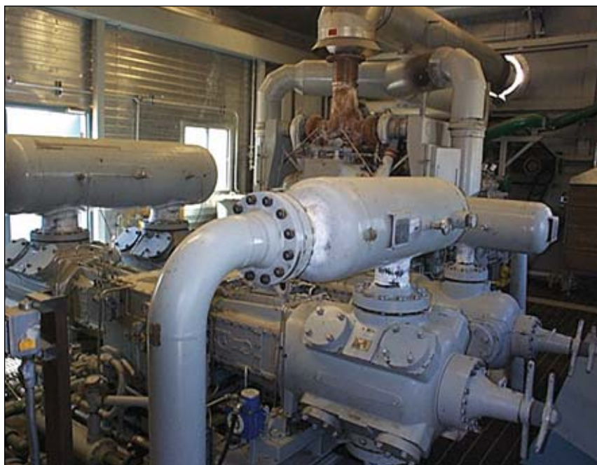
A typical lease package from Hanover Canada. The particular three-stage package includes a Waukesha 5790GL driver (1215 HP) with Ariel JGK/4 compressor, built for up to 2 percent sour service. Hanover has the largest compressor lease fleet at 3.7 million hp worldwide. See the company profile on page B13.
