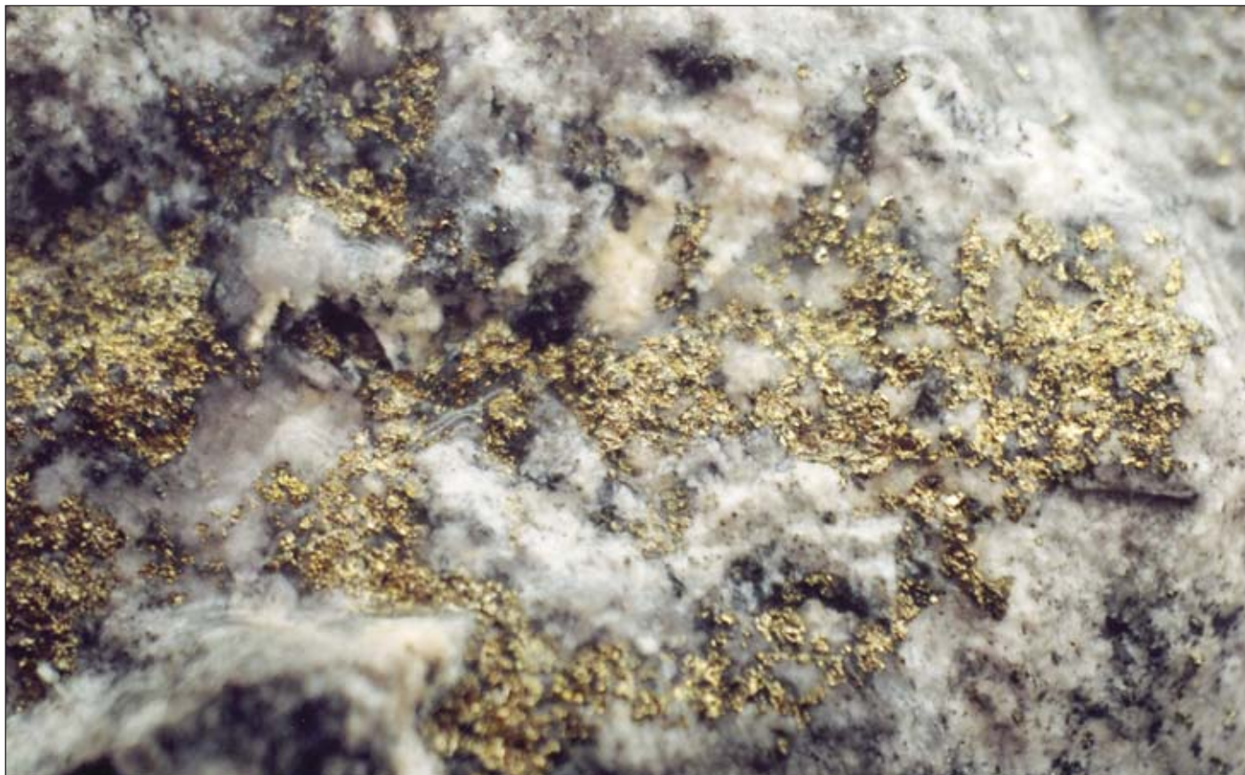
While most of the copper is microscopic in size, some samples are loaded with visible chalcopyrite — copper iron sulfate with a wispy veneer of gold.
