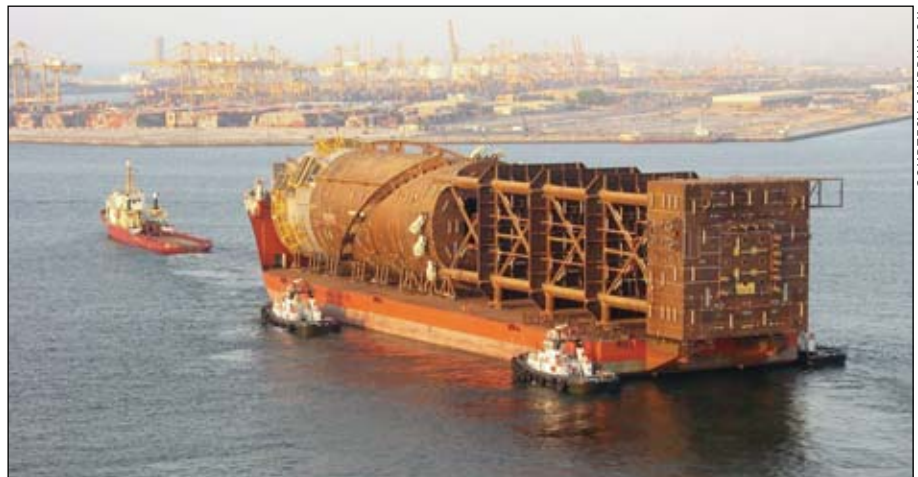
J. Ray McDermott delivered a 14,064 ton truss spar hull in late 2003 for Murphy Oil’s Front Runner project in Green Canyon offshore Louisiana.
