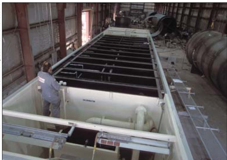
The ALASKAPAK is a water and sewage treatment plant fabricated by STEELFAB for more than 30 years. Ideal for remote locations, and noted for its simplicity and durability, the ALASKAPAK can be fabricated for any size of community and has been popular throughout Alaska. Its flexibility includes anything from basic and safe sewage treatment to providing laundrette and shower components, flush toilets, incineration units and can be linked together for any size of community.
