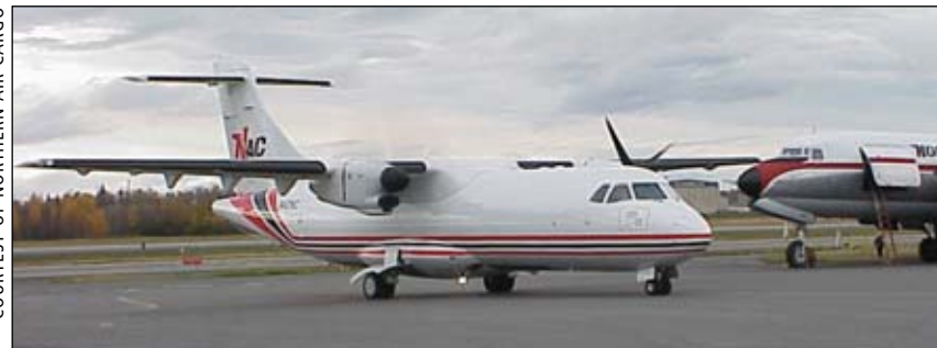
NAC's newest addition, the ATR-42. Because the company's DC-6s are aging, and markets changing, NAC is adding the turboprop ATR-42. Later in the year, two ATR-72s will be added. The air freight company chose the planes for their performance capability, capacity and efficiency.
