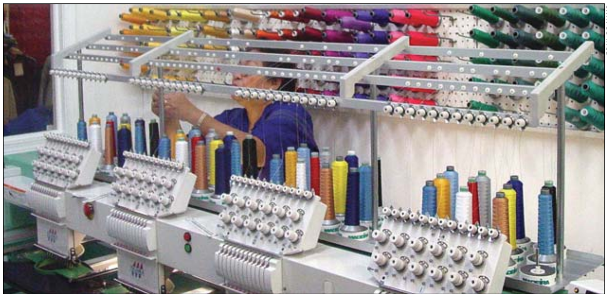
Belen Salazar, 17-year Alaska Textile employee, prepares threads for a custom embroidery job. Digitized software prints out a color-coded threading guide. The machines have the capacity to embroider five items at once.
