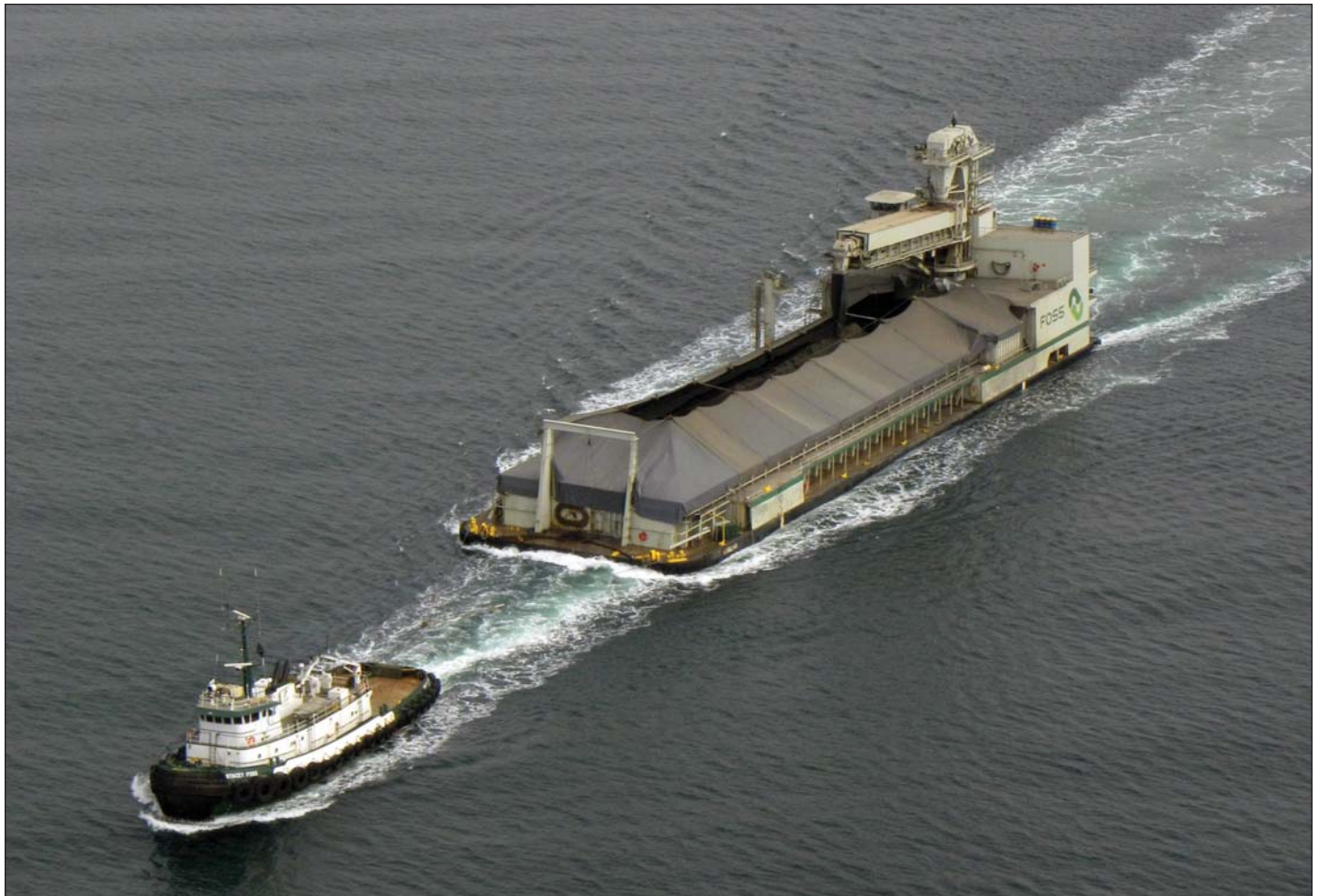
The Stacey Foss tug with Foss Maritime's ore barge, Kivalina, is underway to the Billion Trader near the Red Dog Mine. For the past 18 years, Foss has been a critical link in the transportation and lightering of ore for Red Dog. Foss provides the open ocean lightering of more than 1.4 million tons of zinc and lead ore concentrate to support Teck Resources Ltd.'s operation at Red Dog. For the project, Foss designed specialized equipment, including two self-unloading barges to transport the ore concentrates from the mine's port to ships anchored offshore. With innovative engineering, the company developed the first open-roadstead loading of dry bulk cargo in the world. Courtesy of Foss Maritime Co.
