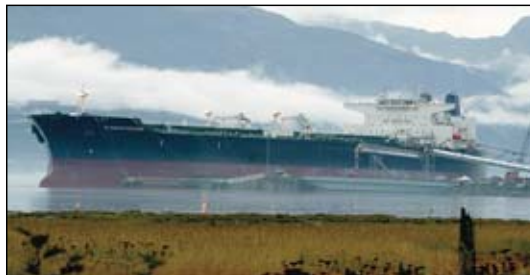
National Steel and Shipbuilding Co., San Diego, made a 2004 delivery of the Alaskan Frontier, first of four Alaska-class double-hull oil tankers being built for BP Oil Shipping Company USA, a subsidiary of BP p.l.c.
