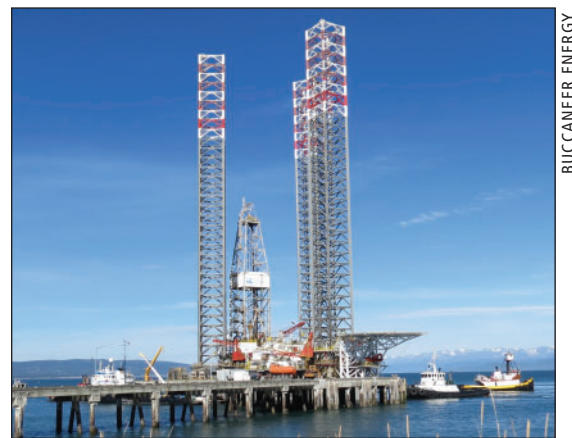
Buccaneer is using its Endeavour jack-up rig to drill the Cosmopolitan well in some 80 feet of water.
