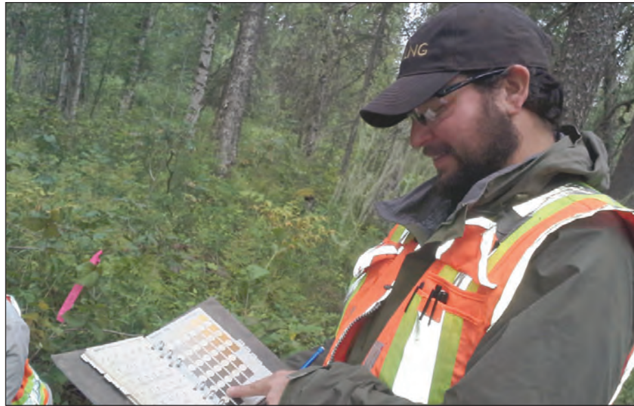
Crew chief Ben Lipke of subcontractor Northern Land Use Research Alaska consults a Munsell soil color chart during a cultural resources study conducted along the proposed Alaska LNG project pipeline route north of Trapper Creek on Aug. 7, 2014. Soil color reveals information about the amount of organic matter, moisture, drainage conditions and the prevalence of minerals in an area.
