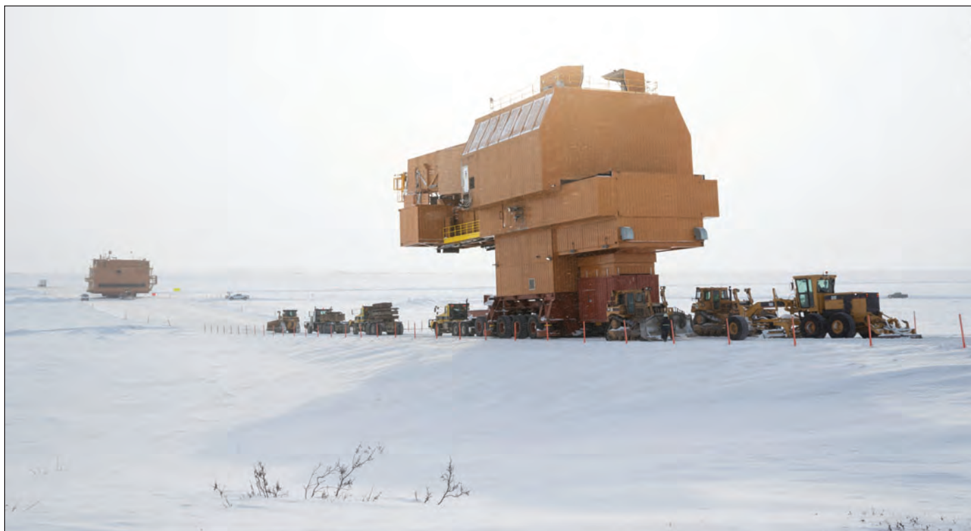
Transportation of a drilling rig on an ice road.
